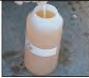
Color: Brown; Severity: 2 Turbidity Severity: 2
