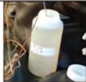
Slight Turbidity Turbidity: 1 (Difficult to interpret this observation; May be natural or an illicit discharge)
