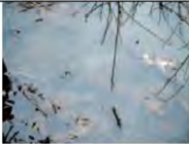
Low Severity Oil Sheen
