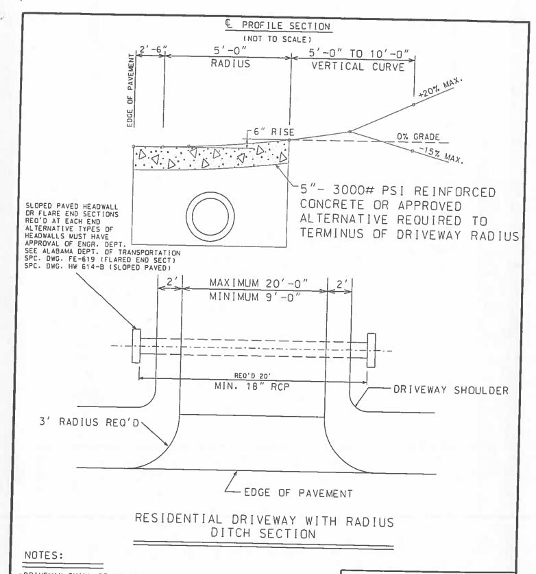
\*DRIVEWAY SHALL BE CONSTRUCTED SO THAT STORM WATER DOES NOT ENTER OR EXIT THE ROADWAY.
